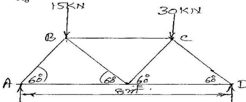
2. Find the forces in all the members of the truss as shown in the figure using method of joints.
