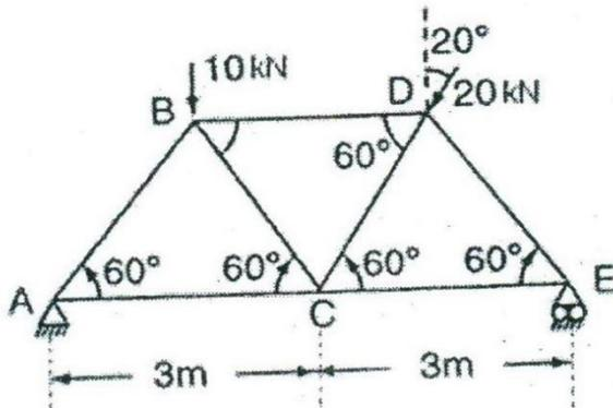
3. Determine the force in member EB of the roof truss shown in the figure. Indicate whether the member is in tension or compression.
