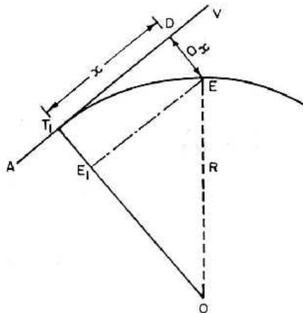
(b) Setting Out By Perpendicular Offsets
