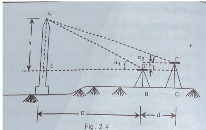
Note: if line of collimation is higher at B than at C, value of  $d$  must be taken as negative.
