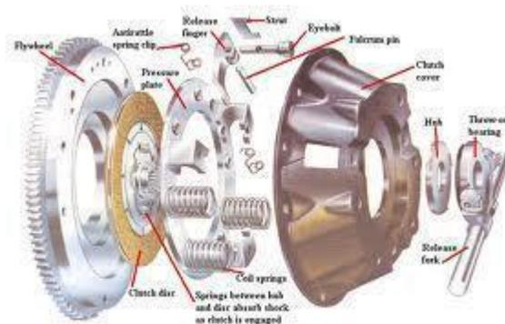
**Fig: Coil Spring Clutch**
